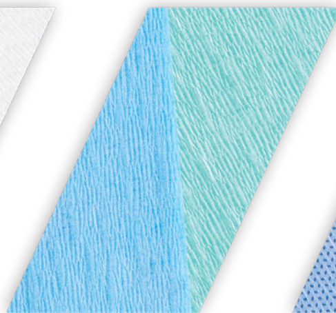
WETLAID NONWOVENS cellulose + synthetic fibers
